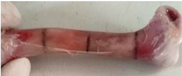
Figure 1. After the measurement, the midpoint was marked as the place where the force would be applied.
